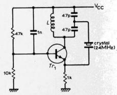
of feedback and the inductor, L, resonates with the series capacitors at the desired output frequency, giving an output which may be taken directly from the emitter resistor or by means of link coupling. The transistor Tr, is a 2N706 (or similar type) and the circuit operates from a 12V supply. L. V. Gibbs.
