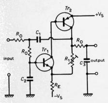
For a ripple of 0.1dB in the pass band and a fall-off of 20dB/octave after cut-off frequency  $f_0$ , choose a convenient value of  $R_0$  and calculate.
