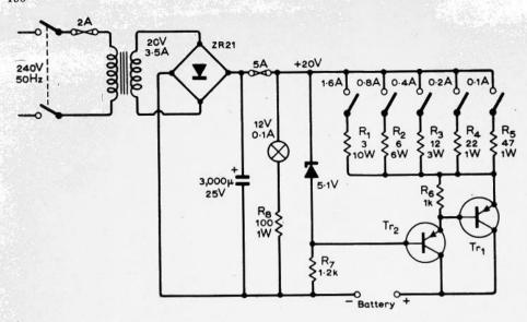
giving a calibrated current which does not alter during charging. Currents from 0.1 to 3.1A may be selected by closing the appropriate switches and the value of current supplied is approximately given by 4.8/R, where R is the appropriate switched resistor. The charging current may be increased to 10A by uprating the selecting different and components values of R.
